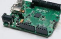
Description: Arduino inspired form factor for VNC2 development. Based on VNC2-64L and includes additional 10-bit ADC
