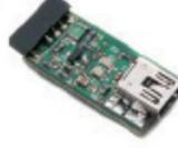
Description: VNC2 Programmer/debugger module for use with the IDE development tools
